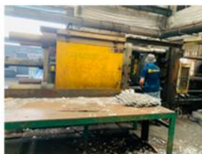
1000 ton die-casting machine
