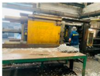
1000 ton die-casting machine
