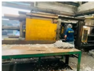
1000 ton die-casting machine
