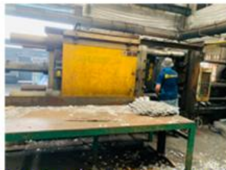
1000 ton die-casting machine
