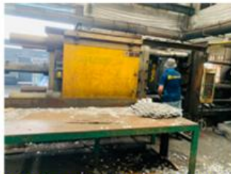
1000 ton die-casting machine
