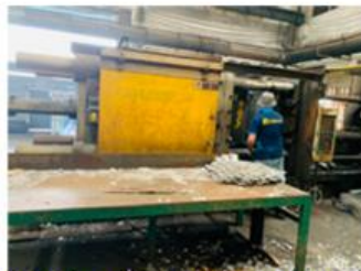
1000 ton die-casting machine
