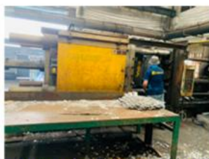
1000 ton die-casting machine
