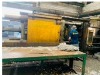
1000 ton die-casting machine
