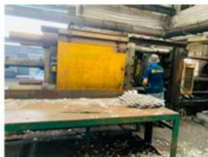
1000 ton die-casting machine
